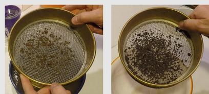
Aggregate stability of tilled silt loam (left) versus a meadow control (right)
